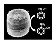
Biosilica structures containing foreign proteins with desired functionalities can be generated by a molecular genetic method. An enzyme immobilized in diatom silica was found to display better activity than purified hydroxylaminobenzene mutase in solution. Such immobilized active biomolecules may find application for the fabrication of sensor materials and reusable catalysts.
