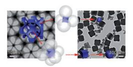
Shipshape: Mesoporous silica nanocubes and spheroids with controllable bimodal size distributions were synthesized within a colloidal crystal template by using a weak acid catalyst to effect the disassem-
