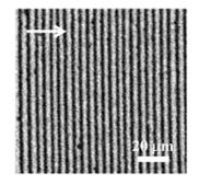
Nanoscience in coffee rings: Nanoparticles with easily tailored optical and electronic properties can be dynamically self-assembled into spatially ordered, 2D patterns (see SEM picture) simply by allowing a drop of a nanoparticle solution to evaporate in a confined, axially symmetric geometry. Utilizing the "coffeering" phenomenon, this approach, which dispenses with the need for lithography and external fields, is fast, cheap, and robust.
