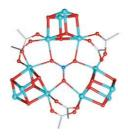
Extraordinary structure: An unprecedented  $Co_{12}$  supercluster in which three  $Co_4O_4$  cubes surround a central  $\mu_6$ -nitrate ligand exhibits single-molecule magnet behavior. The picture shows the structure of the  $Co_{12}$
