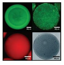
Microgel structures such as spherical microgel shells (picture on the upper left) and spherical microgel particles that incorporate quantum dots, magnetic nanoparticles, and polymer microparticles (other images) have been prepared by a capillary microfluidic technique. Because these particles change their volume with changes in temperature, they may find application in, for example, drug delivery.
